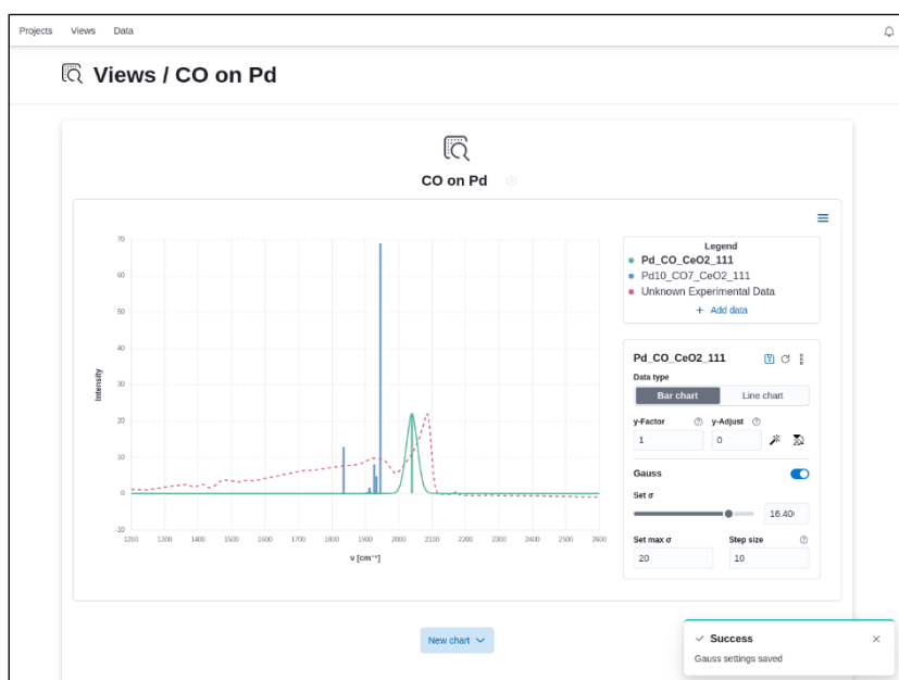
Figure 1: Comparison between several simulated and experimental IR spectra. Gaussian widening is applied to one of the DFT spectra.
